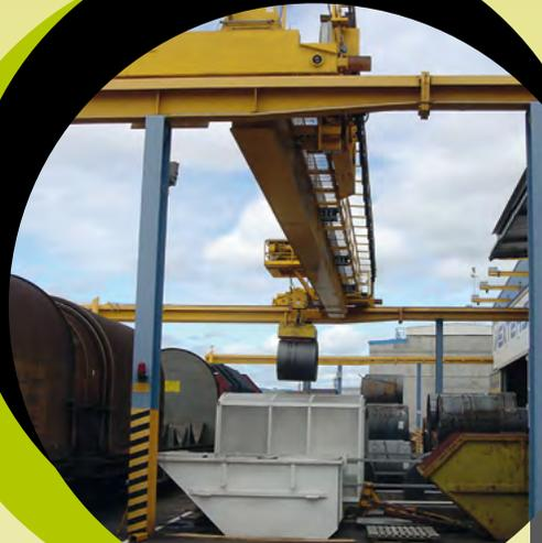
*Gauss Magneti has also successfully developed the electropermanent magnets technology. Electropermanent magnets hold their magnetization also in case of net failure or cable break, so they do not need buffer batteries or mechanical safety forks.*
