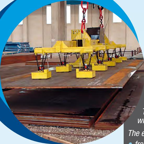
*The magnets can be used individually, multiple under a fixed or an extensible beam allowing the magnets distance to be adjusted according to the plates dimensions. These electromagnets can also be used for handling packs with iron hoops able to stand the load.*
