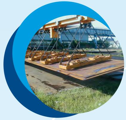
*GAUSS MAGNETI designs and manufactures since 1972 special rectangular electromagnets for plates and packs, keeping into account the customer strong requirements for optimal managing of the available space in plant, for high movements speed and for possibility to handle one or more plates at the same time*
