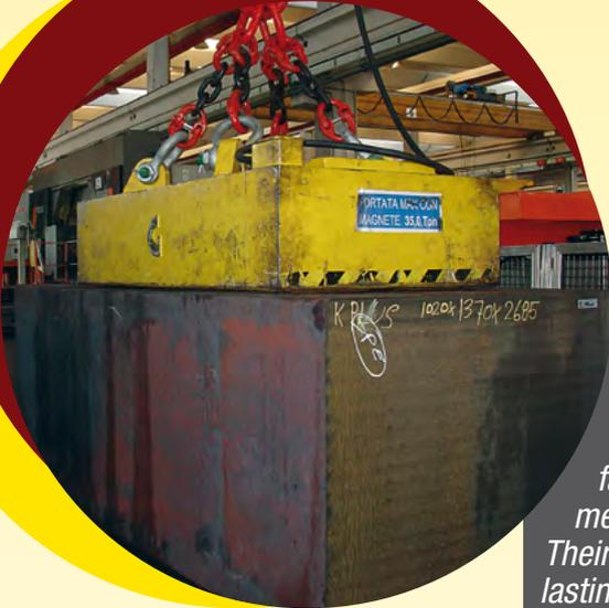
*Gauss Magneti has also successfully developed the electropermanent magnets technology. Electropermanent magnets hold their magnetization also in case of mains failure or cable break, so they do not need buffer batteries or mechanical safety forks.*
