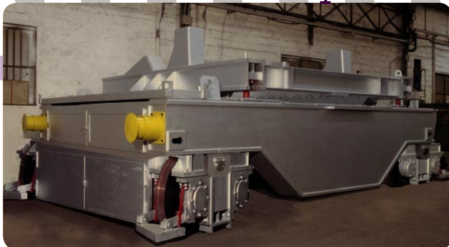
I Carro per siviere UK Coil transfer for ladle F Chariot transfer de récipient de coulée D Gießpfanneabwagen
